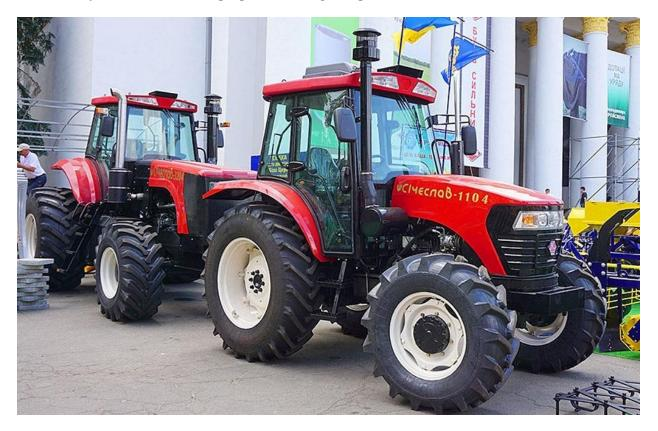
Let's start with the wheeled tractor "Sicheslav-1104". It is equipped with 4-cylinder diesel engine Deutz WP4T110E200 with power 110 hp (430 Nm for 1400 - 1600 rpm). Transmission - mechanical, 16 transmission - forward, 8 - back. Fuel consumption - 195 g/kWh. Capacity of fuel tank - 150 l. Total length with front load - 4330 mm, width - 2080 mm, cab height (with air conditioning) - 3120 mm. Road clearance - 380 mm.
