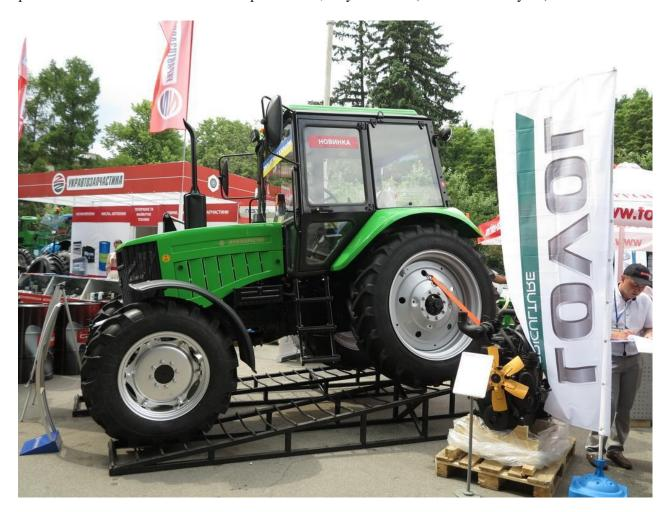
The tractor got another design of the front part. The enlarged radiator grill holes minimize the possibility of overheating the engine. By the way, the motor is installed more powerful, turbo-charged - 105-strong D-245-174. The headlights of the European model moved to the top. Transmission - 18-step, with the possibility of hidroponyzhuvalnoho gear, which increases the number of transfers twice.
